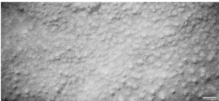
Fig. 2. Upper surface of ion-etched polyimide membrane. The bar represents 1000 Å.
